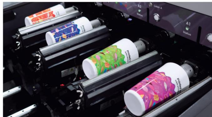
4 different files can be output simultaneously on 2 × 2 operation stations
