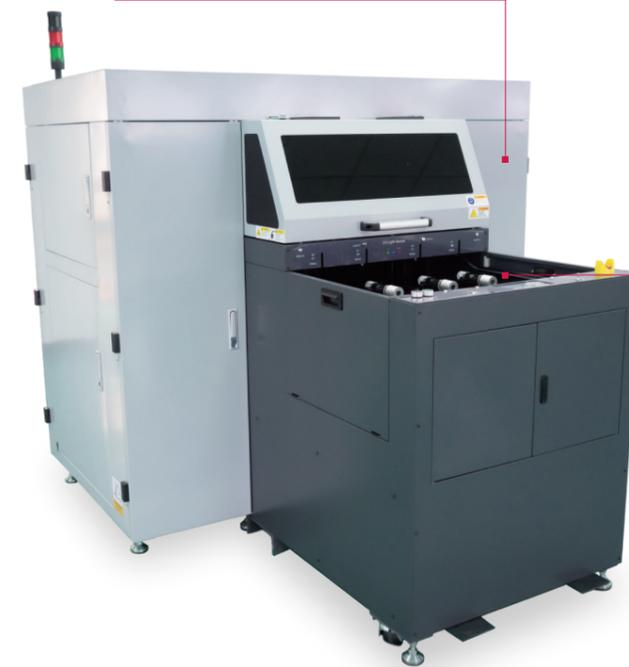
Based on an all-in-one design concept, the small and compact **Print Head Maintenance Module** allows automatic purging, wiping and capping for convenient unattended operation.
