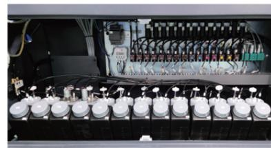
**Automatic ink supply system** monitors and controls ink levels of the main and sub ink tanks with liquid level sensors. (The above photo for 11-channel model)
