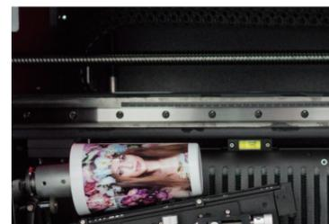
**Positioning Sensors** indicate the position of the print object and enable to quickly set the printing area, achieving efficient and precise printing.
